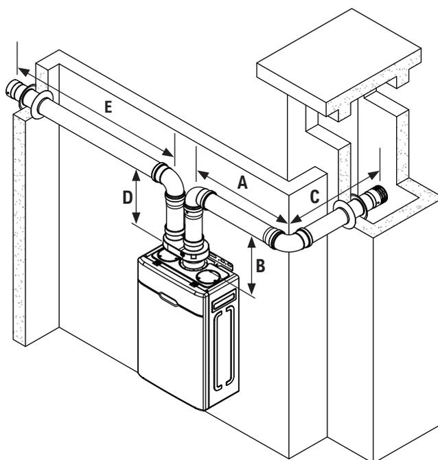
$$15 - (3 \times \text{колено } 90^\circ) = 12 - (3 \times 2,0) = 12 - 6 = 6 \text{ м}$$
